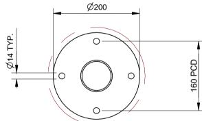
Detail A **BOLT DOWN DETAIL TIMBERS & CASTING** HIDDEN FOR CLARRITY
